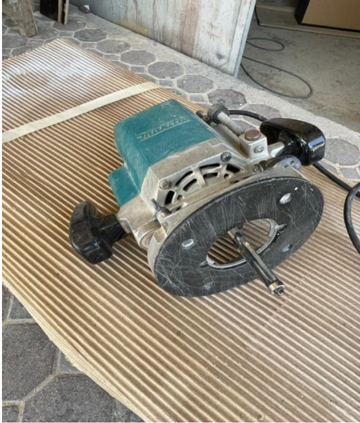
Router for hollowing out parts for weight reduction
