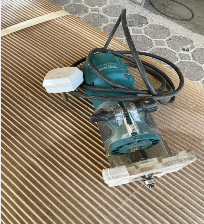
Trimmer for rounding the edges
